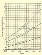
Fig. 253.—Prime movers used in central stations.\*
